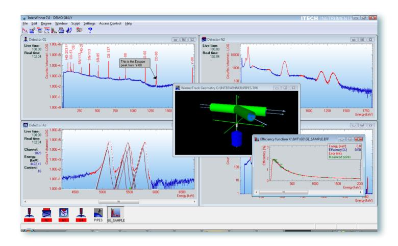
**InterWinner 7.0** is a universal nuclear spectroscopy analytical program simultaneously controlling up to 32 inputs. **InterWinner** provides different analysis engines for Germanium, NaI, LaBr and CZT based gamma spectroscopy as well as solid state Alpha spectroscopy. **InterWinner** is available in versions to support several or all of these detector types.
