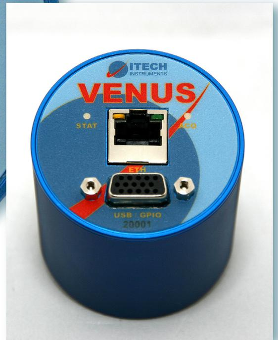
The **Venus** is a universal digital multichannel analyzer integrated into a photomultiplier base. The **Venus** can be used in the most exacting spectroscopic applications as well as high rate, industrial counting applications. Because of our range of user selectable gain and time constant options, the **Venus** is easily adapted to all of today's choices of scintillator, including NaI, CsI and LaBr.
